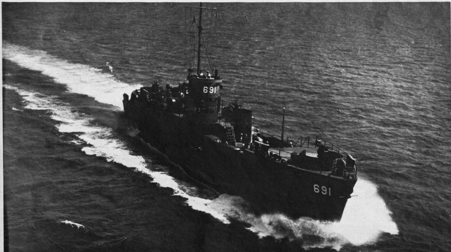
Recognition features of LCI(L) are easily seen here. Rounded bridge shows craft to be a newer model. Lack of side ramps is the conspicu-
